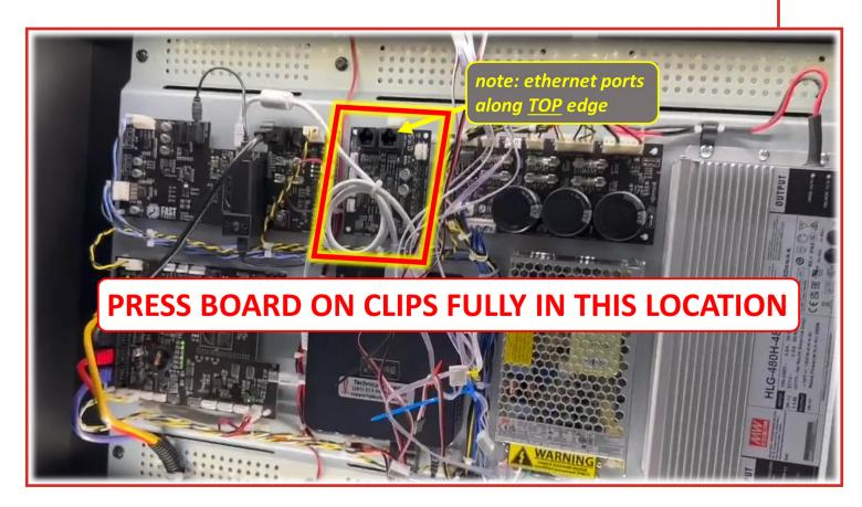
7. Use the provided cables to connect the circuit board to the existing game circuit boards as show below
